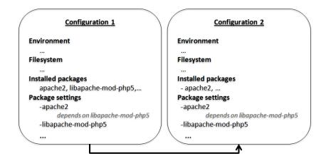
Fig. 7. Incorrect package removal
